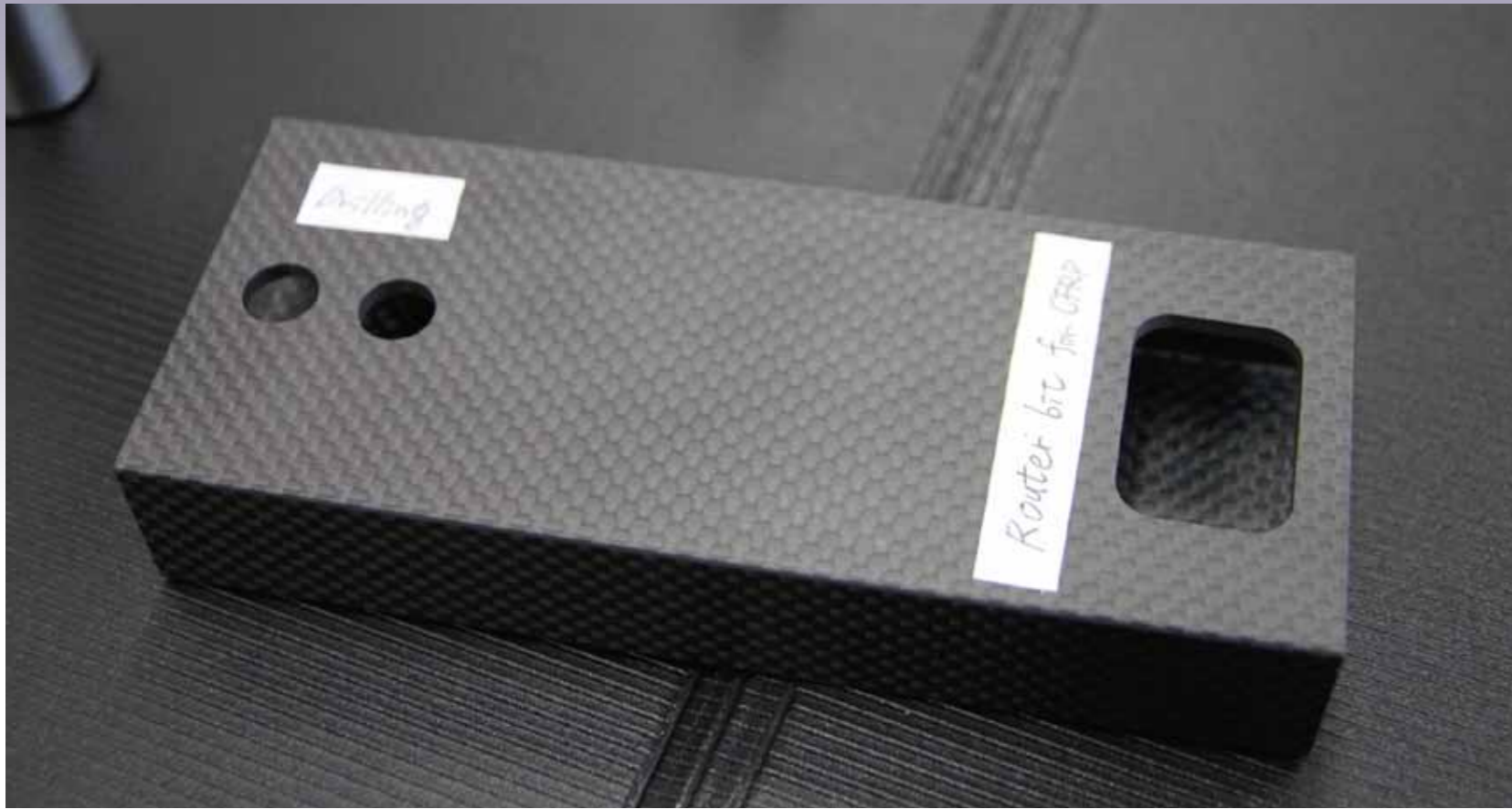
Cutting test (CFRP)
