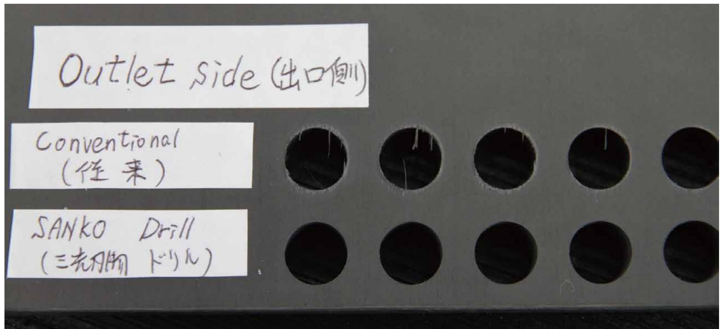
Drilling test (Outlet side of the CFRP-UD)
